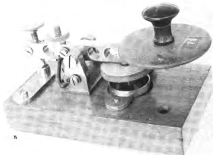
● (75) Ducretet & Rogers, Paris. (Oil break key with contact at bottom of well shown under lever arm)
